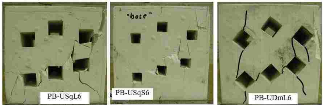
Figure (4.41) Photographs of Tested Cubes Containing Unisize Non-circular Voids
