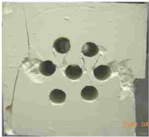
a- Tension Failure (Vertical to sub-vertical fractures)
