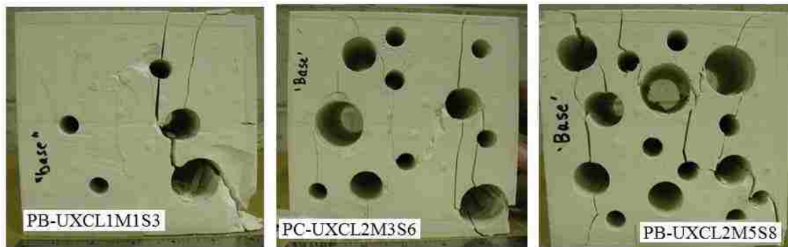
Figure (4.34) Photographs of Tested Cubes Containing Mixed Circular Voids
